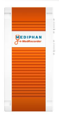
Mediphan MedRecorder™ is a simple solution for the capture, archive, organization, and retrieval of diagnostic-quality medical images and DICOM images from nearly any medical device that has a video display (VGA or DVI). It is an effective low-volume picture archive and communication system (PACS) solution, and can also be used to enhance hospital security.
